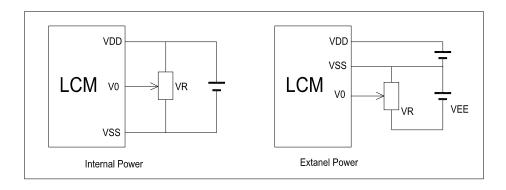
$V_{DD^{\sim}}V_0\text{: LCD Driving voltage}$
